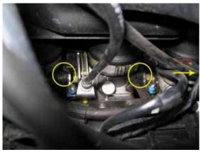
The springs aren't heavily wound. What we'll be doing is moving the end from position #1 to position #2.
