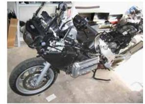
Pictured here is the left side of the engine, after gas tank removal, but prior to airbox removal. The throttle bodies and springs are located on in there somewhere. It may look scary, but don't be afraid.
